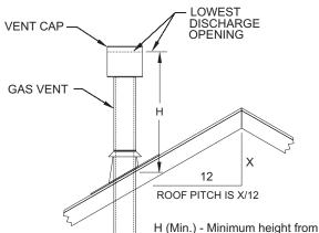
H (Min.) - Minimum height from roof to lowest discharge opening
